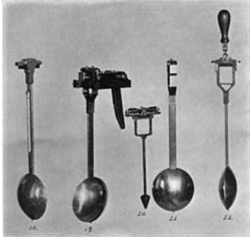
Pendulums used in Mendenhall gravimeter, 1890
