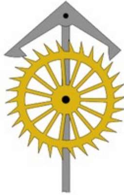
Animation of anchor escapement , one of the most widely used escapements in pendulum clocks
